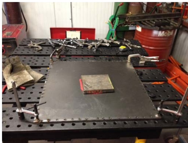
Figure 6 : Welding Sheet Metal
